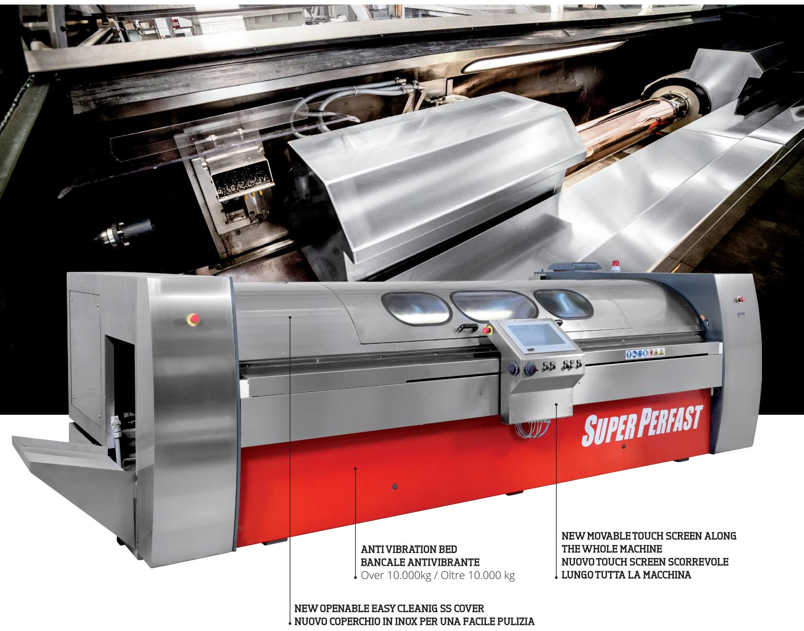
Acigraf proudly present the only real simultaneous cutting and polishing machine for rotogravure cylinder Super Perfast.
